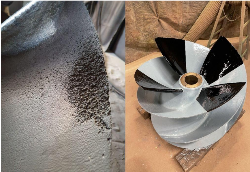
Cooling water pump impeller repaired and protected against cavitation. Image credit: ISEA d.o.o.
